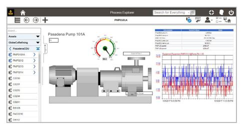
With the help of aspenONE Process Explorer, Aspen IP.21 enables combining navigation with an asset symbol and its historical and real-time data.
