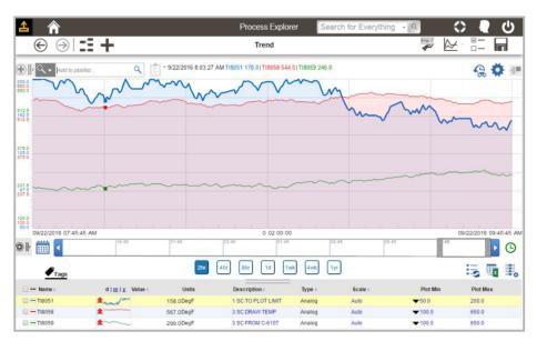
With the help of Aspen IP.21 and aspenONE Process Explorer, users are able to monitor the performance of plant equipment and navigate through their historical and real-time data.
