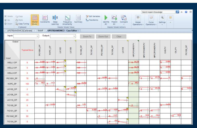
Figure 6: DMC3 model matrix combining linear, linearized (via transforms) and full nonlinear deep learning variables.
