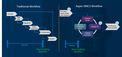
Figure 4: Traditional vs DMC3-enabled APC methodologies.
