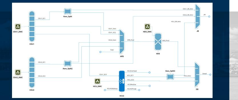
Figure 8: Aspen GDOT flow sheet with templated, Hybrid and APC models integration.
