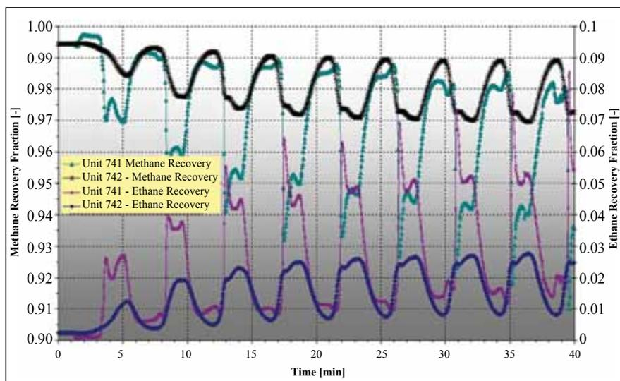
Figure 5: Oscillatory column behaviour with an overall master pressure control
