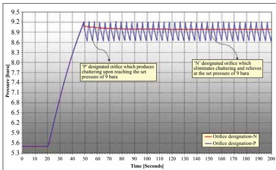
**Figure 1: PSV upstream pressure variation: comparison between a steady PSV discharge flow and flow during PSV chattering**
