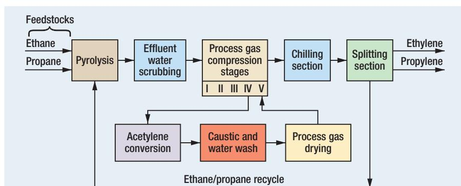
FIG. 2 Process flow diagram of Olefins I plant.
