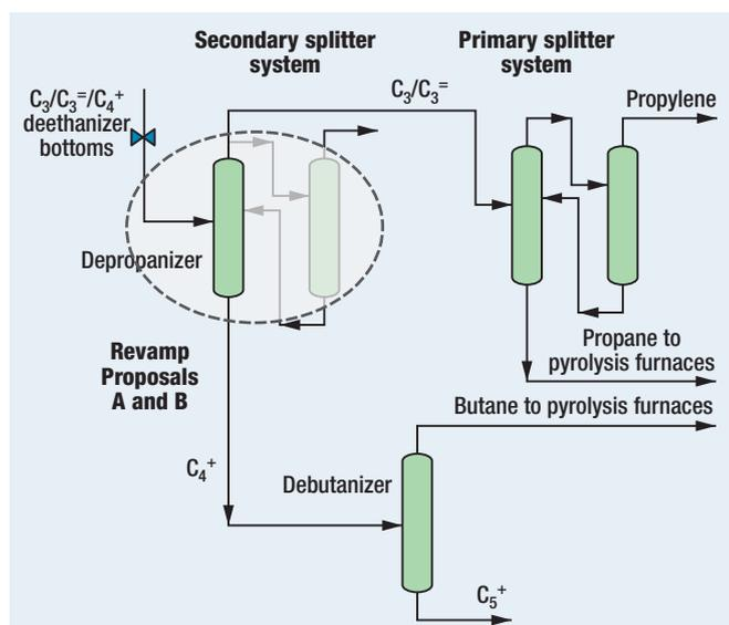
**FIG. 6** Proposals A and B: Use one column in the secondary C<sub>3</sub> splitter as a depropanizer.
