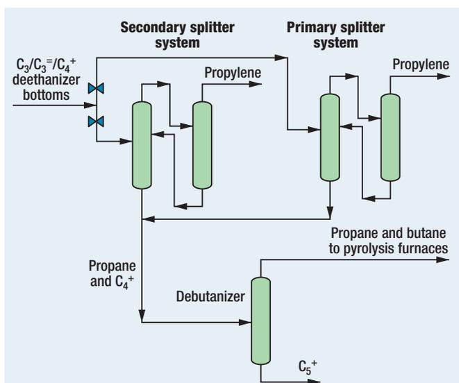
FIG. 4 Propane/propylene splitter section of the existing unit.
