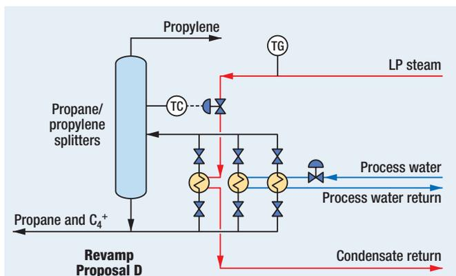
**FIG. 8** Proposal D: Using LP steam as the heating medium in reboilers.
