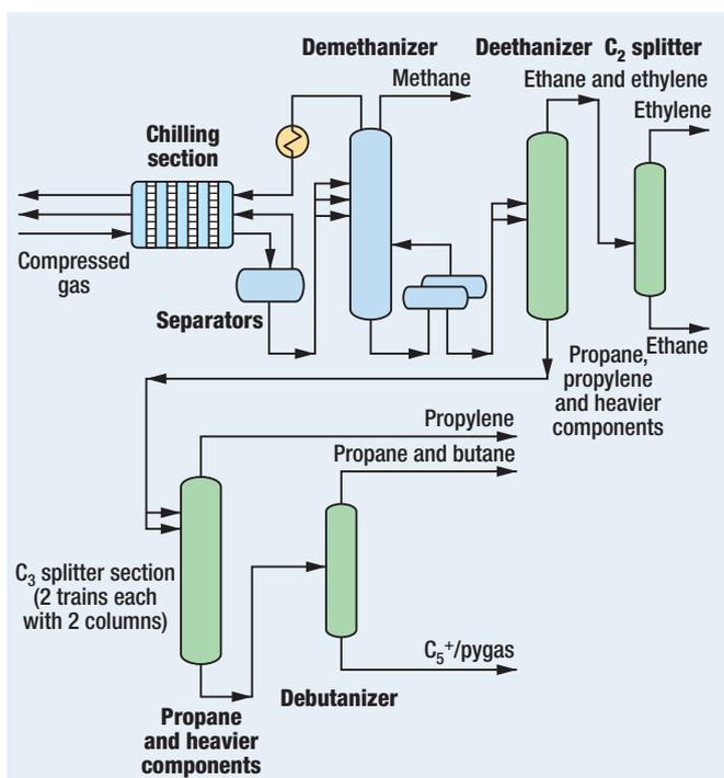
FIG. 3 Separation section of the Olefins I plant.
