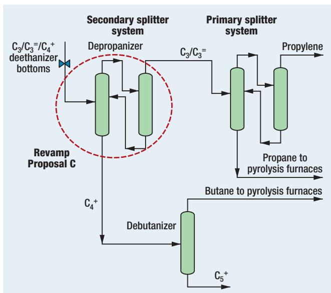
**FIG. 7** Proposal C: Use the secondary splitter system as a depropanizer.
