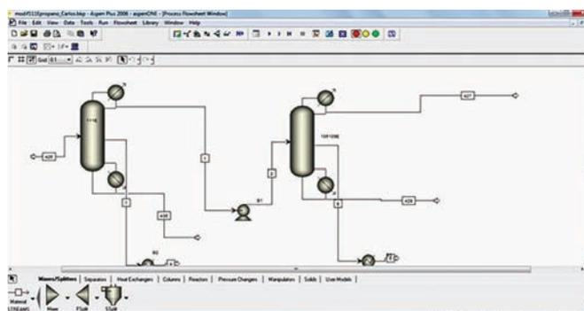
**FIG. 5** Simulation model of the propane/propylene splitter system.
